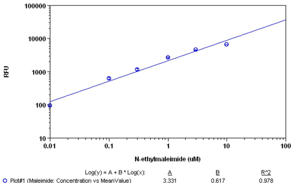
**Figure 1.** N-ethylmaleimide dose response was measured in a 96-well black plate with Amplite™ Fluorimetric Maleimide Quantitation Assay Kit using a NOVOstar microplate reader (BMG Labtech). As low as 0.1 μM (10 picomol/well) of maleimide can be detected with 10 minutes incubation time (n=3).
