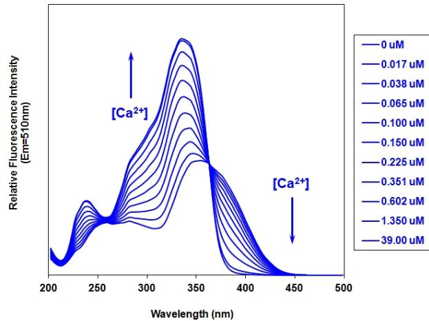
**Figure 1.** Fluorescence excitation spectra of Fura-2 in solutions containing 0 to 39uM free Ca<sup>2+</sup>.
